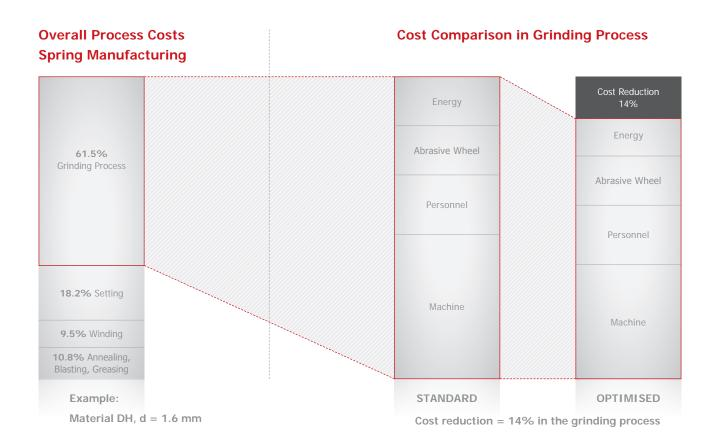
If, as a precondition, grinding results of consistent quality are being achieved, the grinding process can be optimised by shortening the machining time and/or processing time, reducing the set-up times and lengthening the dressing intervals. These three points interact with each other and cannot be considered separately. However, it can be achieved: by using optimised abrasive wheels, you increase the spring throughput per time unit. **This will enable you to reduce your process costs.**
